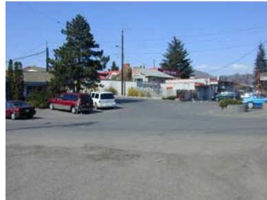
From Oak Road intersection (west leg) looking North to Elm Road. The large area of unmarked pavement and uncontrolled access creates a very large conflict area close to Tranquille Road
